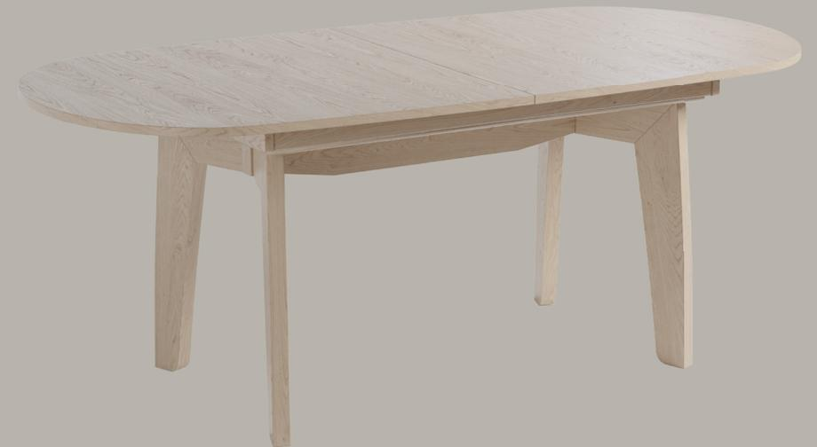
When you pull one of the end of the tabletop, the additional leaf pops up from the magazine, you unfold the two parts of the leaf, and finally you push the tabletop back.
